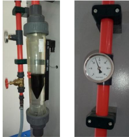
**Picture 2. Thermometer and rotameter indicators**
